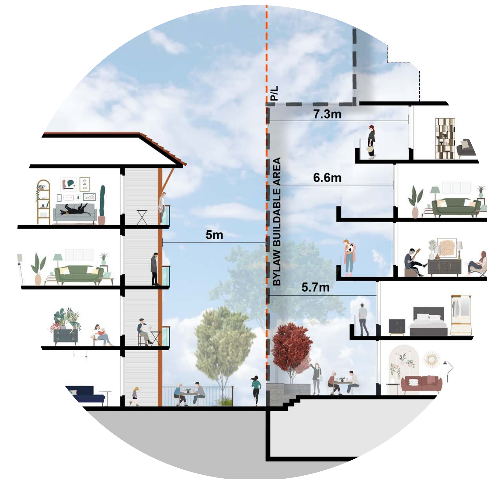
Section of The Vintage at Waterscapes with Waterscapes Phase 1 to the west Top - Towers T1 and T2 interface plan; Bottom - Towers T3 and T4
